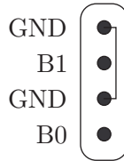
Figure 8. Analog outputs connector CON3.
